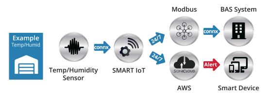
This example shows a sensor transmitting temperature and humidity data 24/7 in a warehouse to the SMART IoT meter, which sends it to the BAS system and the SoniCloud platform simultaneously. Users receive alerts on their smart device if user-set temperature or humidity limits are exceeded in the warehouse. You can also connect equipment to your BAS/BMS system using RS485, dry-contact, or custom protocols.
