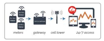
900 MHz gateways that transmit by 4G/5G LTE to the SoniCloud cloud-based platform. Cellular transmission is over an encrypted VPN connection for maximum security.
