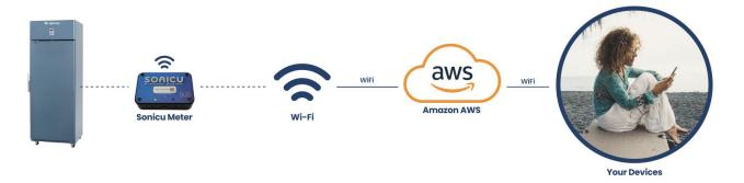
Sonicu Duo meters can be equipped with Wi-Fi radios configured to communicate with the Client's WiFi network. This option allows the client to use an existing WiFi infrastructure to add meters anywhere the Wi-Fi network is accessible.
