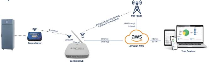
Data is transmitted via Duo meters using SoniLink Hubs that are connected via Ethernet. The hub uses the client network to send data to SoniCloud.
