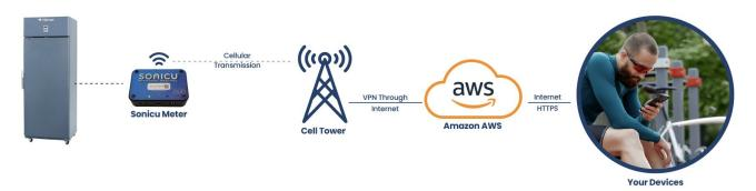
Most Sonicu Duo meters can serve both as the meter and a data gateway by using a cellular modem internal to the meter.
