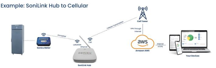
Sonicu's Duo meters sit in the client facility and never use the client's internal network. Sensor data is transmitted via Duo meters to a central cellular SoniLink Hub and then to Sonicu's AWS platform.
