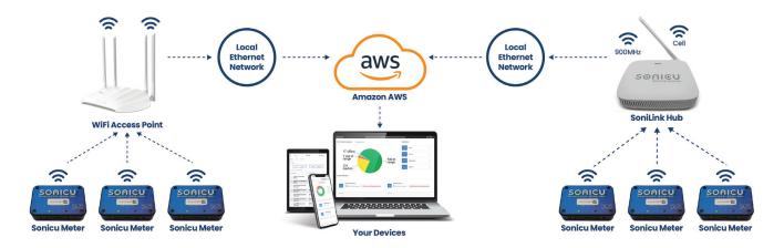
Optional 900MHz meters provide a boosted signal that can run either **ON** or **OFF** network via a Gateway. The gateway transmits to the cloud via Ethernet, 4G LTE, or Ethernet with 4G Failover. Refer to the diagrams to choose the option that is best for your organization. Contact a Sonicu sales representative for assistance.
