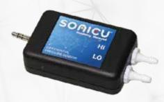
**Digital Differential Air Pressure Sensor** – Simple plug-and-play deployment with accuracy of +/- .25% and range of +/- 4-inches water column. Easily connects to a variety of pickups that include air duct mounts, wall plate or ceiling mount applications.
