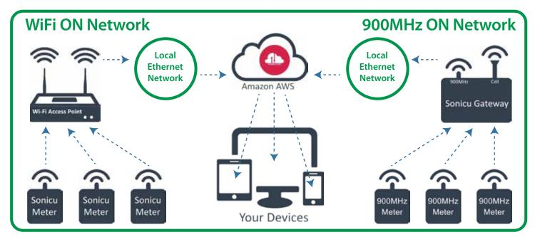
Optional 900MHz meters provide a boosted signal that can run either **ON** or **OFF** network via a Gateway. The gateway transmits to the cloud via Ethernet, 4G LTE, or Ethernet with 4G Failover. Refer to the diagrams to choose the option that is best for your organization. Contact a Sonicu sales representative for assistance.
